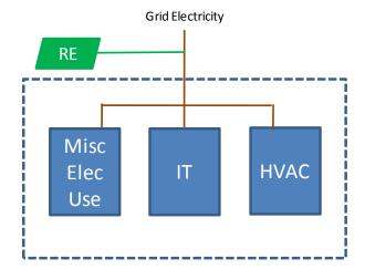
Figure 1: Data center PUE calculation boundary with renewable energy
