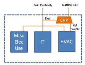
Figure 2: Data center PUE calculation boundary with CHP.
