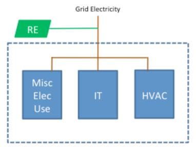
Figure 2: Data center PUE calculation boundary with renewable energy
