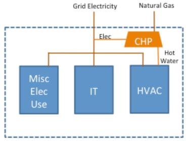
Figure 3: Data center PUE calculation boundary with CHP.
